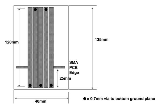
Material: Double-sided FR4 0.0625" 2oz copper, ENIG, Er=4.2 @ 300Mhz flooded ground on bottom side Resonators are 5mm wide, with 0.7mm gap, 120mm long Input/output lines are 2.47mm with edge-mount SMA PCB
