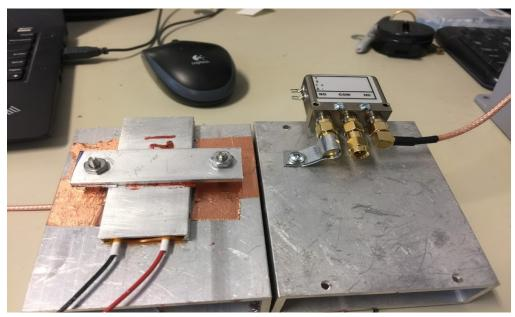
Two of the "thermal stages" are shown above. The PTC heater resides on the bottom, and the RF relay on the edge of the top. The 500hm terminator is strapped to the stage itself, to improve thermal transfer/stability, and the LNA will be connected to the middle, "common" port on the relay. The "sky" signal arrives on the short SMA terminated cable coming in from the right.
