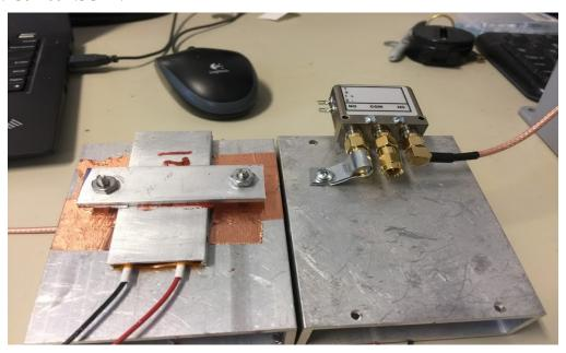
Two of the "thermal stages" are shown above. The PTC heater resides on the bottom, and the RF relay on the edge of the top. The 50Ohm terminator is strapped to the stage itself, to improve thermal transfer/stability, and the LNA will be connected to the middle, "common" port on the relay. The "sky" signal arrives on the short SMA terminated cable coming in from the right.
