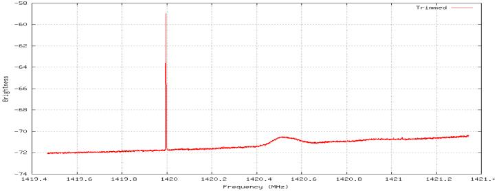
This has nicely eliminated the "edge roll-off", but we still have a narrow-band artifact (in this case, from the receiver itself) at exactly 1420 MHz (the 142<sup>nd</sup> harmonic of the 10MHz reference clock). It's also important to note that there's an obvious "passband slope" in this plot, which is, again, an instrumentation artifact.
