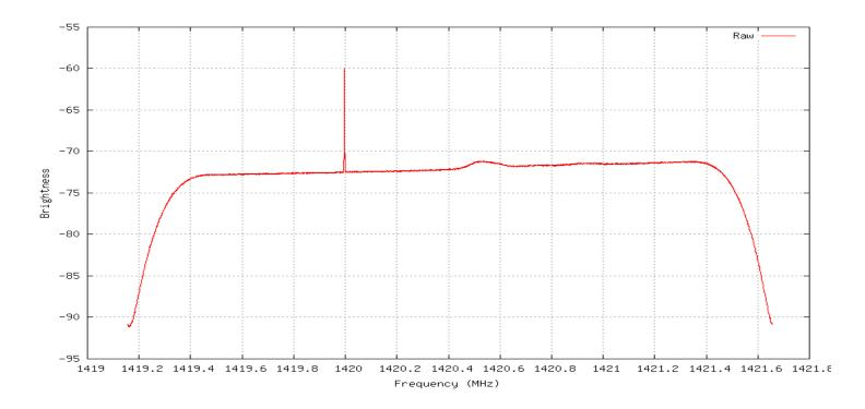
It is immediately obvious that there are some artifacts that must be dealt with in order to proceed with further processing. This processing is performed using the "makepixels.py" tool in the *maptools* package. The edges of the plot fall-off steeply, which is to be expected with any band-limited signal, so our first job is to reduce the "view" to eliminate the "edge roll-off":
