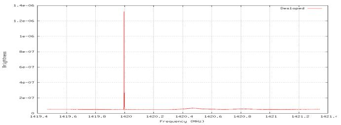
Next the data are conveted into a temperature profile, given some calibration constants based on receiver characteristics, and large excursions above the minimum are removed (removing the spike at 1420MHz, or at least reducing it to inconsequential levels).
