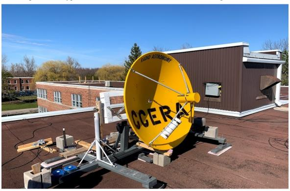
The feed is connected to an off-the shelf Low Noise Amplifier (LNA) assembly, providing approximately 40dB of sub-0.7dB NF gain. The LNA was provided by *NooElec*<sup>1</sup> as a prototype
