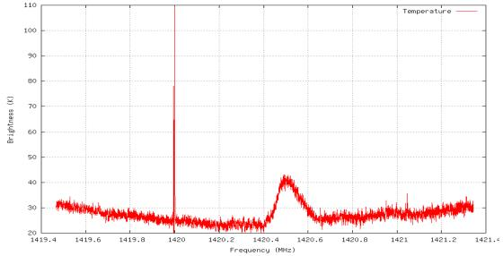
Here we can see the data have been converted to Kelvin, and the spike at 1420 is quite a bit smaller than it otherwise would have been.
