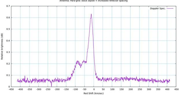
Doppler Specturm: RA 20.5 DEC+45, Fc=1420.406M, BW=6M Antenna: Para-grid: stock dipole + increased reflector spacing
