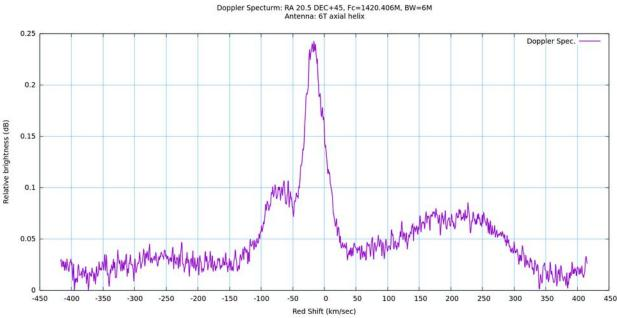
The SNR is poor, and the peak sky response is a paltry 0.25dB above the noise.
