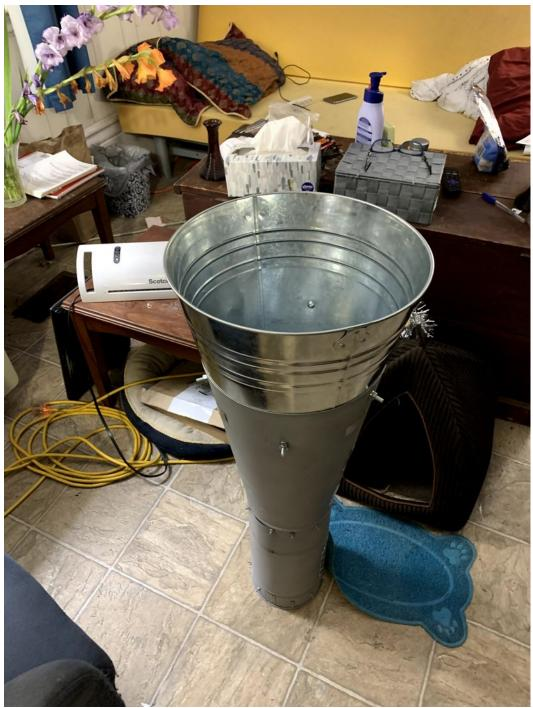
The CAD\$9.00 bucket was modified by cutting out the bottom and fitting it to the existing somewhat-smaller circular-horn antenna.
