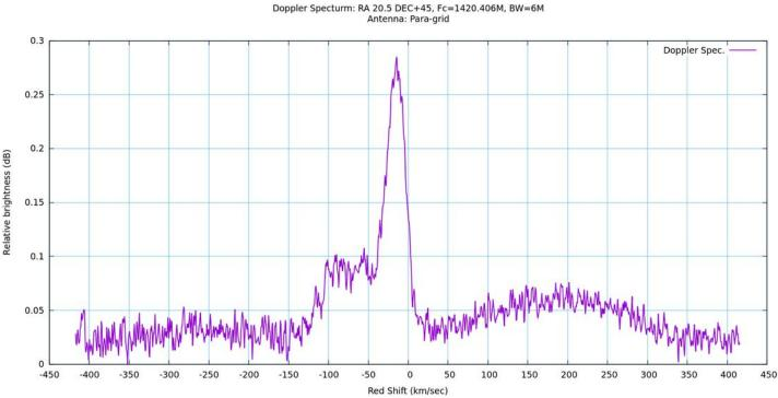
This was certainly adequate for an initial observation, but theoretically (given the effective aperture of this 30cm x 60cm parabola) the response should have been better.
