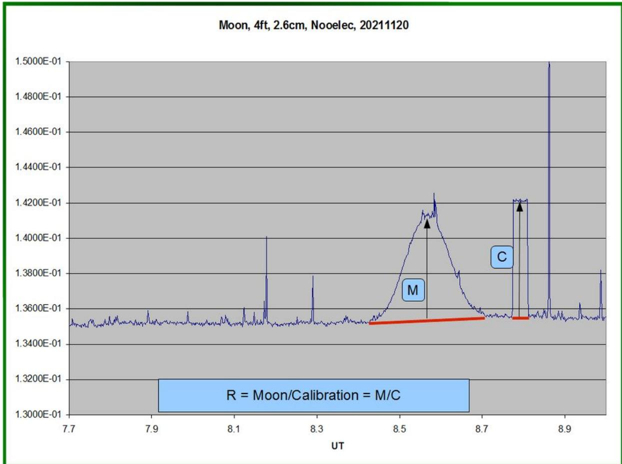
Figure 8: Method of measurement. Note the baseline change during the lunar transit. The implicit assumption is that the change during the transit was linear. This is a possible cause of error.
