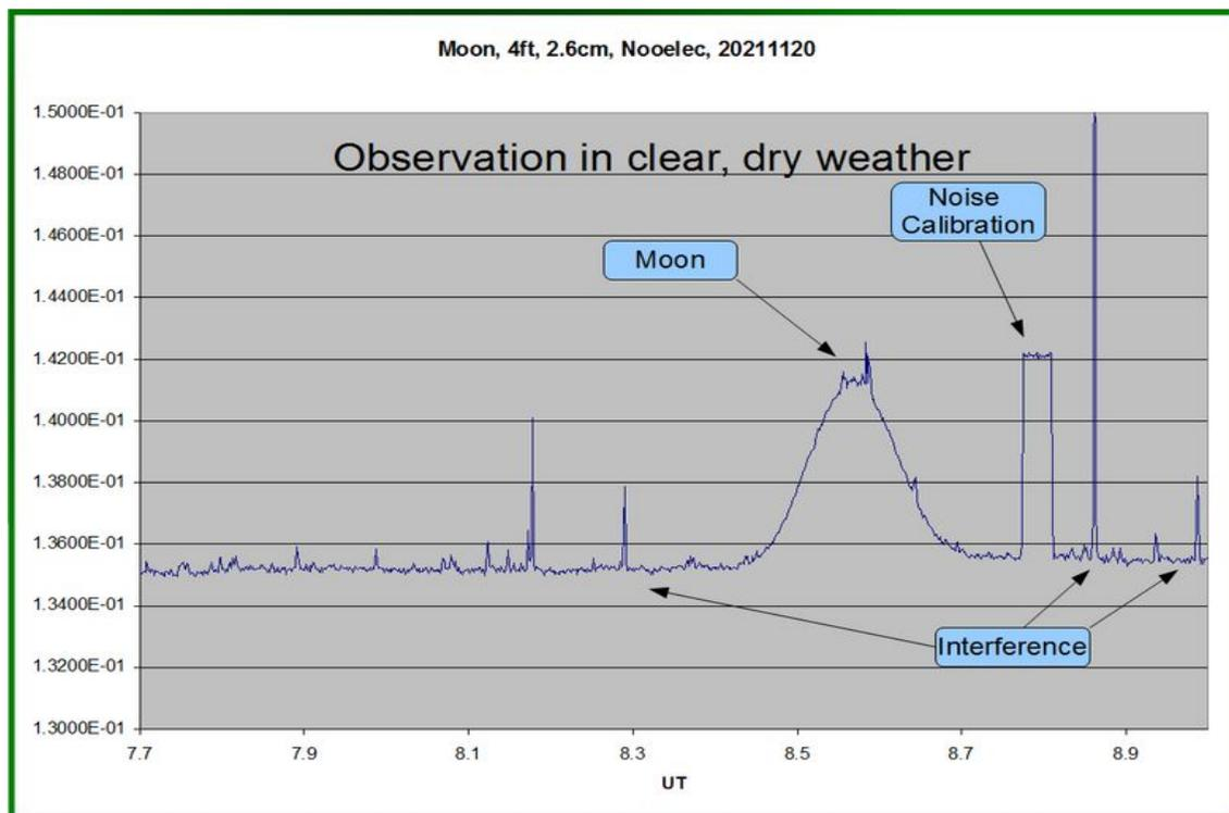
Figure 5: An example of a lunar transit as recorded with the 1.2m dish.
