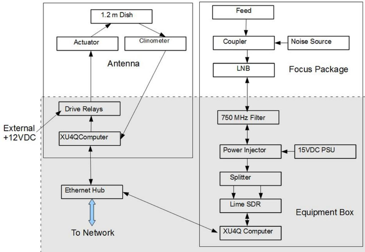
Figure 4: System Block Diagram. Components in the shaded grey box are located in the equipment box
