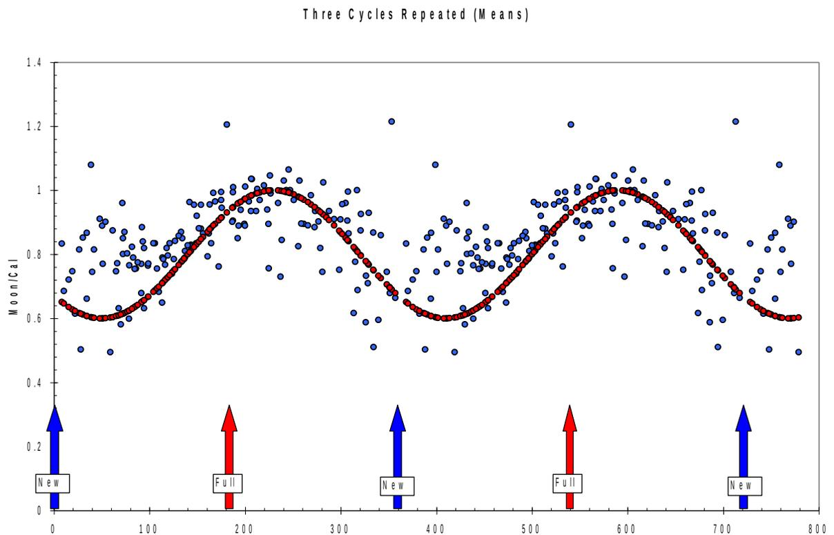
Figure 10: Mean Daily values repeated to show the variation more clearly. The fitted sinusoids is not a model, just a tool for identifying the day of peak radio brightness temperature, which is about 2.5 days after Full Moon. Horizontal axis is UT hours.
