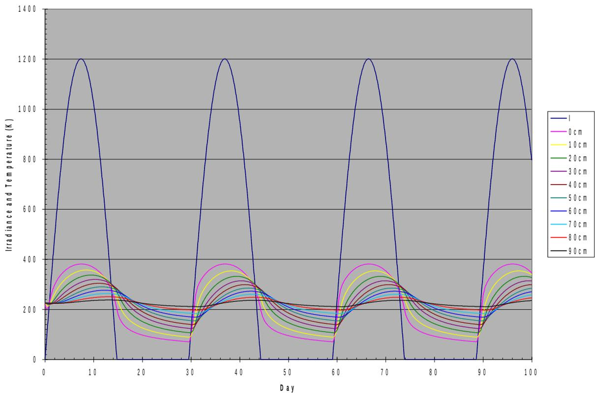
*Figure 11: Heat input and modelled subsurface temperature changes in every tenth of the 100 layers as a function of lunar phase.*
