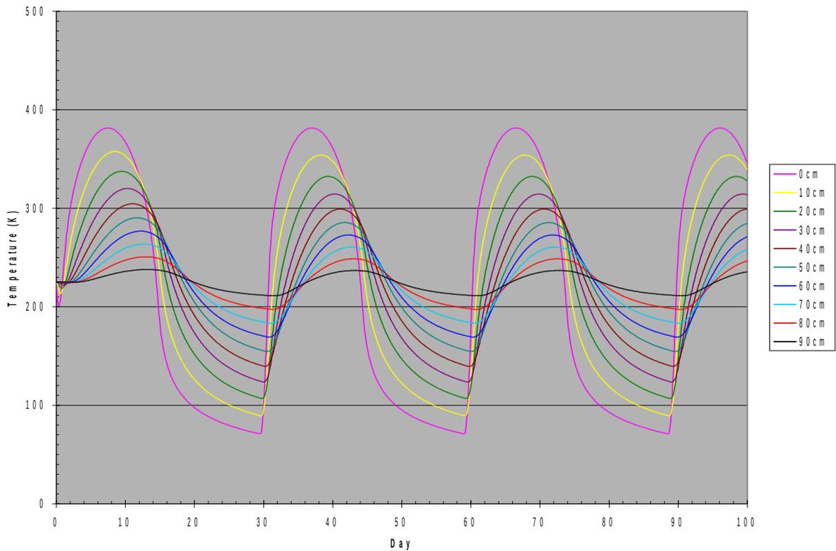
Figure 12: Temperatures as a function of depth and time. The phase lag with increasing depth is clearly visible.
