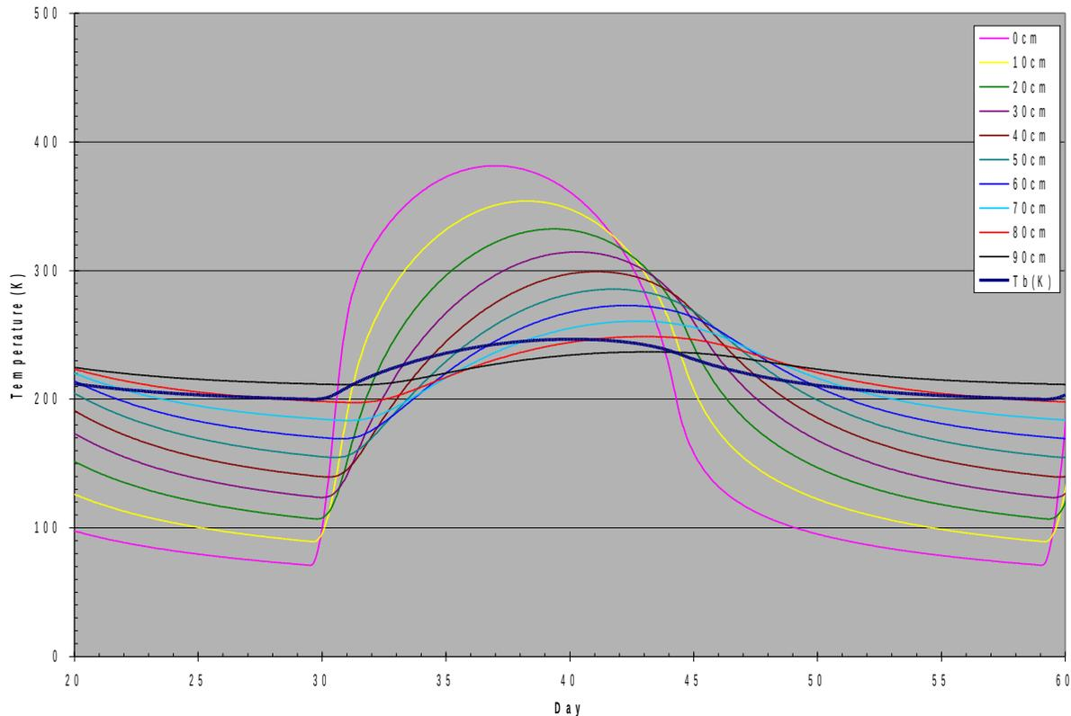
*Figure 13: One cycle, showing the temperature variations as a function of depth and time, and the modelled radio brightness temperature (thick, black curve). There is a delay of about 2.5 days between the peak temperature at the surface and the peak radio brightness temperature at 2.6cm wavelength.*
