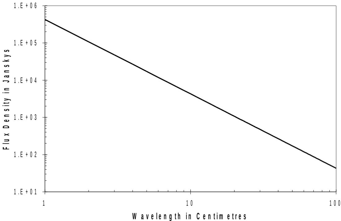
Figure 3: The approximate radio emission spectrum of the Moon. The line shows the flux density of the lunar emission as a function of wavelength. A Jansky is  $10^{-26} \cdot \text{w} \cdot \text{m}^{-2} \cdot \text{Hz}^{-1}$ .
