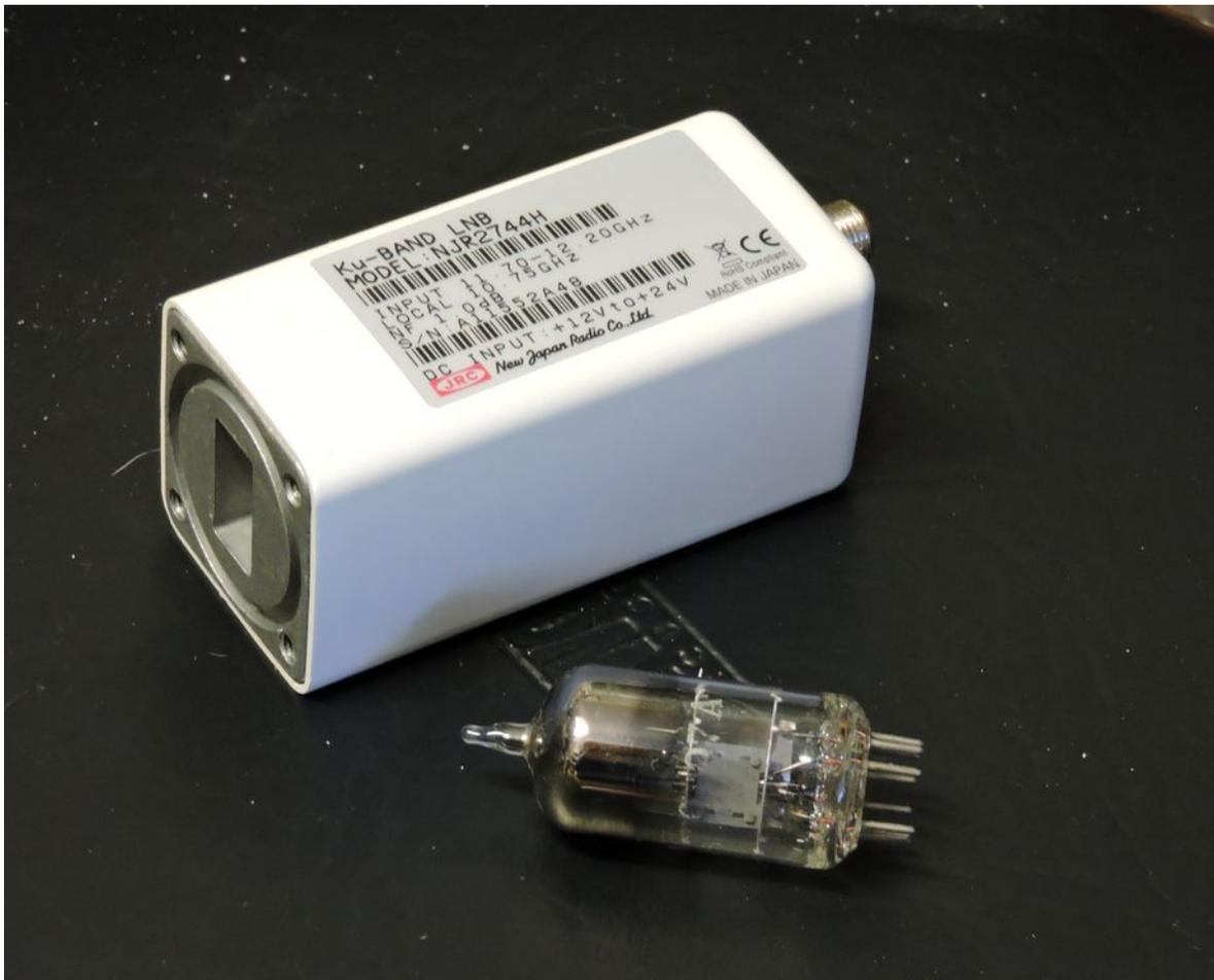
*Figure 1: The Ku-Band block downconverter used for this project. An older style amplification device is included for comparison purposes.*
