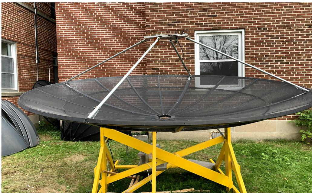
course in astrophysics. The target pulsar is “bright” at lower frequencies, which means that an antenna with quite-modest gain is required to observe it. Indeed many amateurs now routinely observe J0332+5434 with a more-modest antenna than we use at CCERA. Our antenna, (shown above) is a 3m mesh parabolic reflector, with a full-wave loop feed. It provides more than enough antenna area to realize our observing goal.
